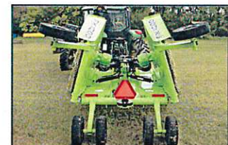
Narrow transport over-centering wing design
