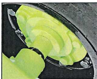
Metal seal guards on 517 hubs
